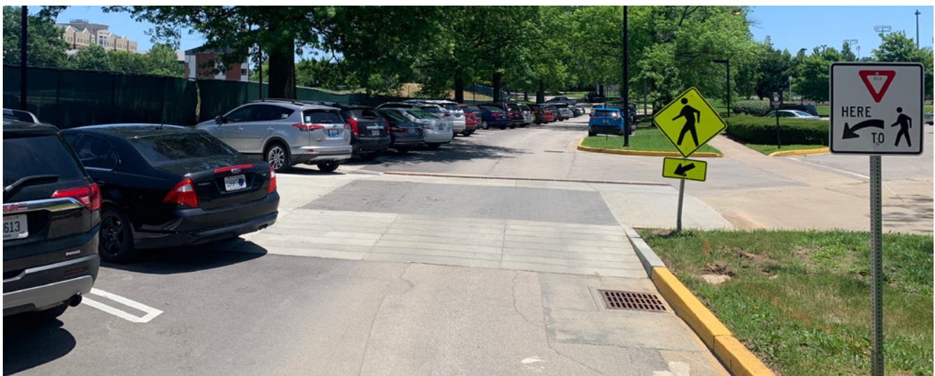
Figure 5.8 Complex Drive raised crosswalk and angle parking
