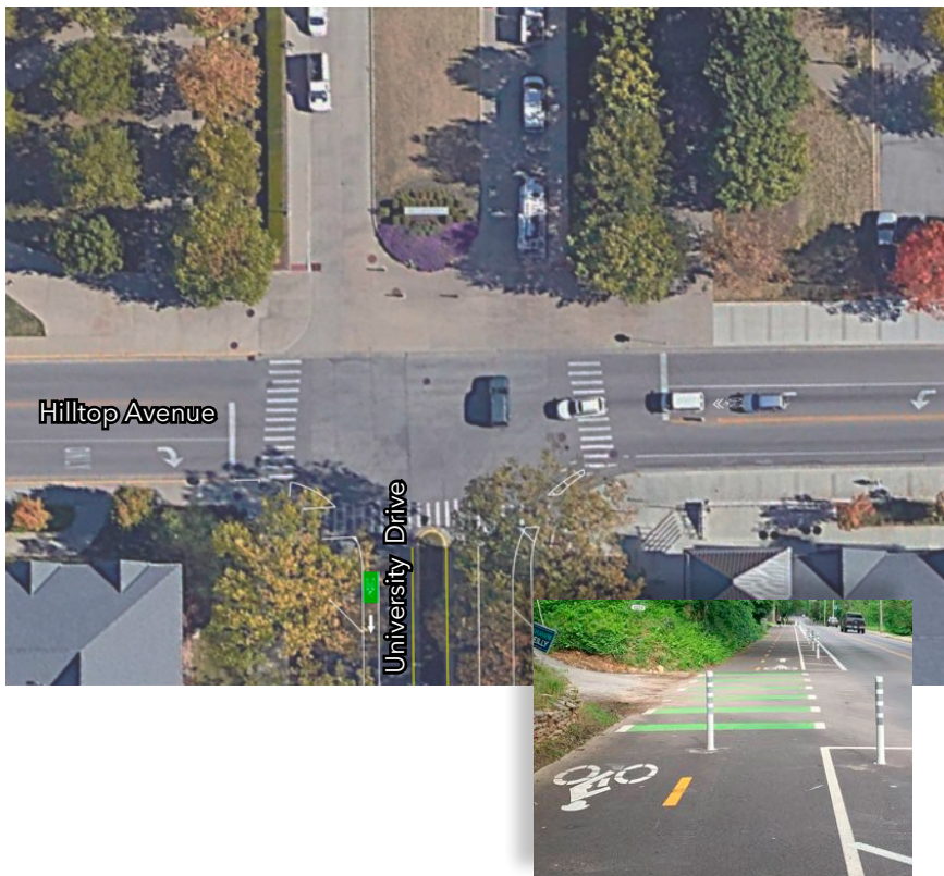
Figure 5.29 Protected intersection for right turning bicyclists at University Drive and Hilltop Avenue, featuring buffers like those shown in the inset.
