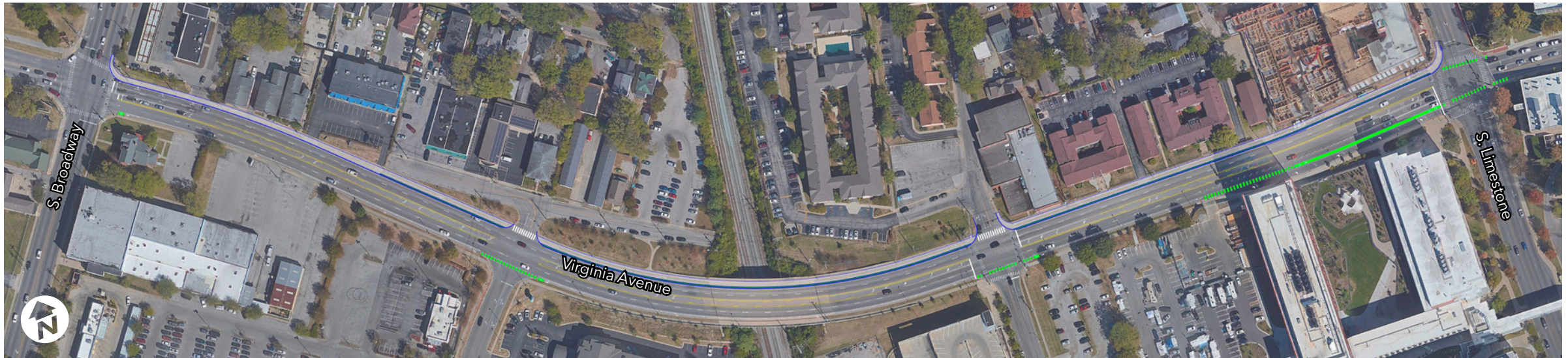
Figure 5.49 Proposed north side shared use path along Virginia Avenue, with a buffered eastbound bicycle lane on the south side.
