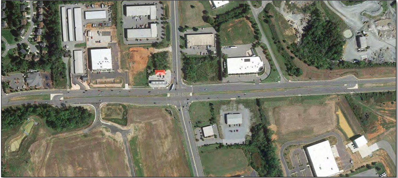
Figure A5.2 - Median U-Turn Example from FHWA
