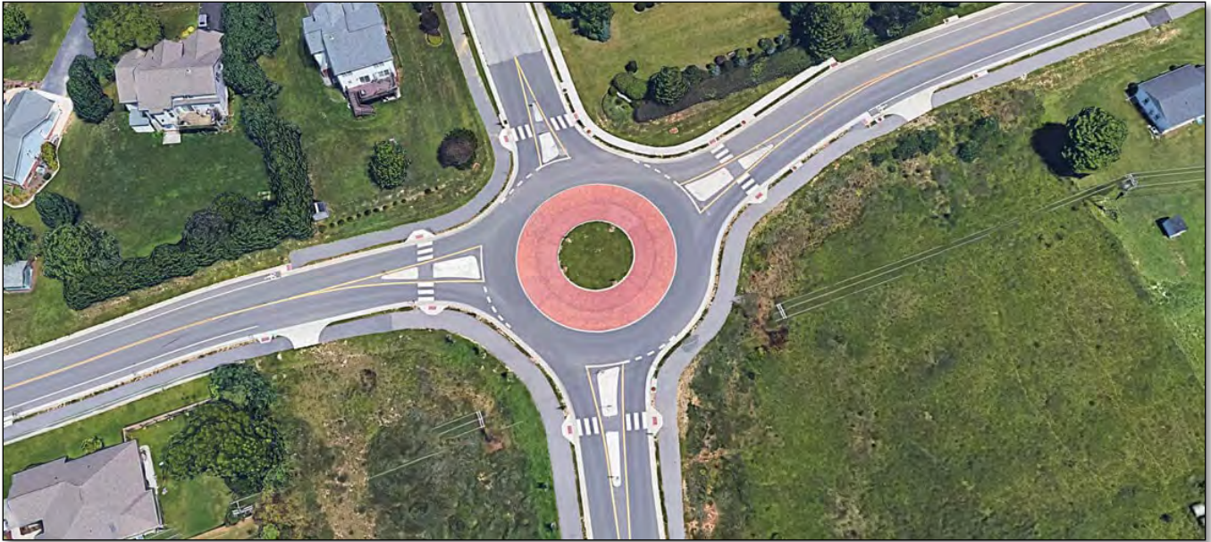
Figure A5.3 - Single Lane Roundabout Example, FHWA
